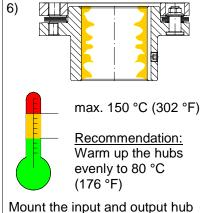
Check and prepare the shafts and hubs for mounting: apply lubricant (see Chapter 8.3).
