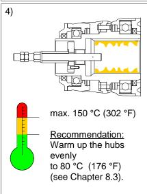
5) Mounting the T type coupling with mounting device (Chapter 8.3).
