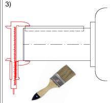
Check and prepare the shafts and hubs for mounting: apply lubricant (see Chapter 8.2).
